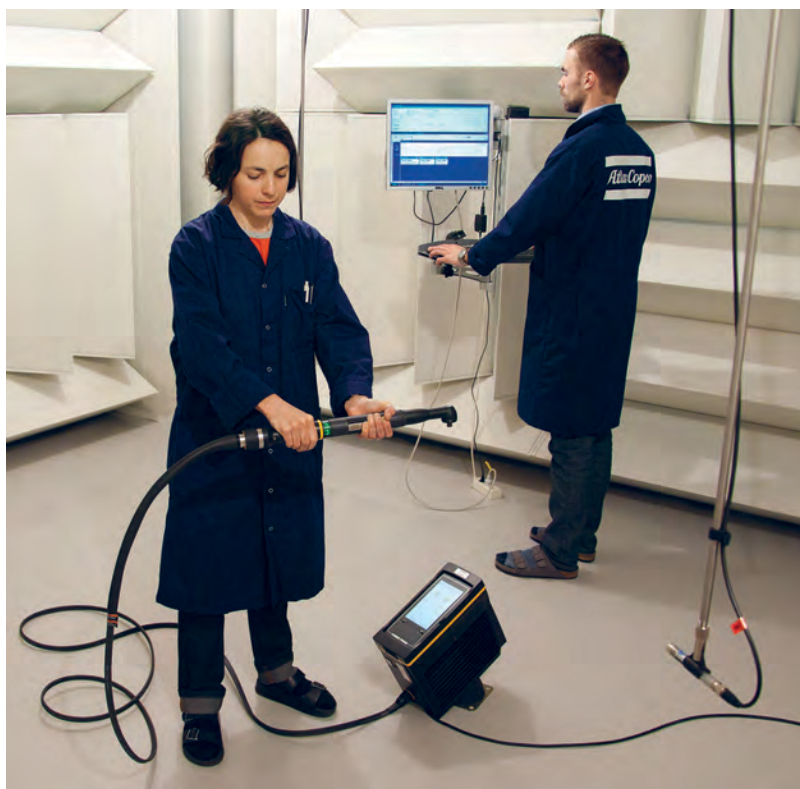
Atlas Copco has a well equipped laboratory for measuring tool noise and vibration emissions. It contains advanced vibration measurement tools, a state-of-the-art acoustics laboratory and dedicated computer software for analysing measurement and test results.
